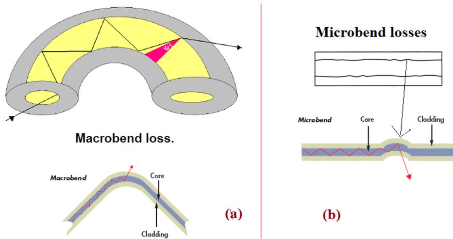
Figure 17: macro bending and micro bending losses
