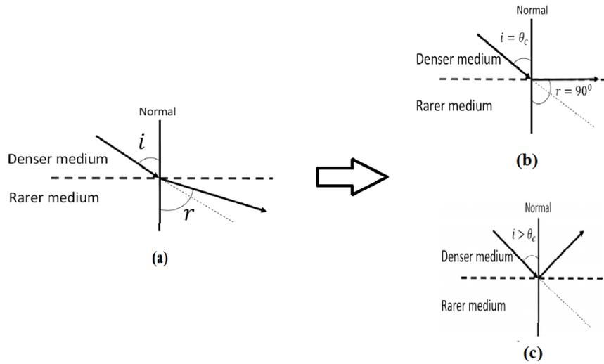
**Figure 10:** Total internal reflection
