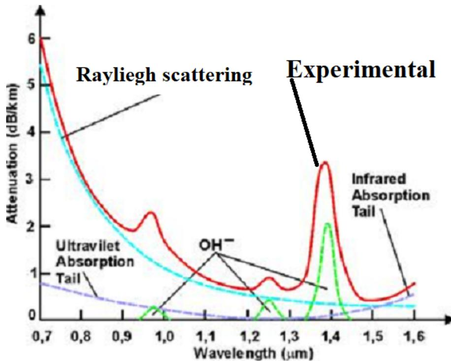
**Figure 16:** Attenuation in optical fiber
