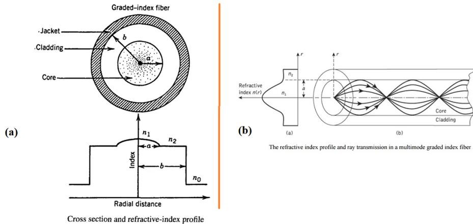
**Figure 15:** Graded index fiber
