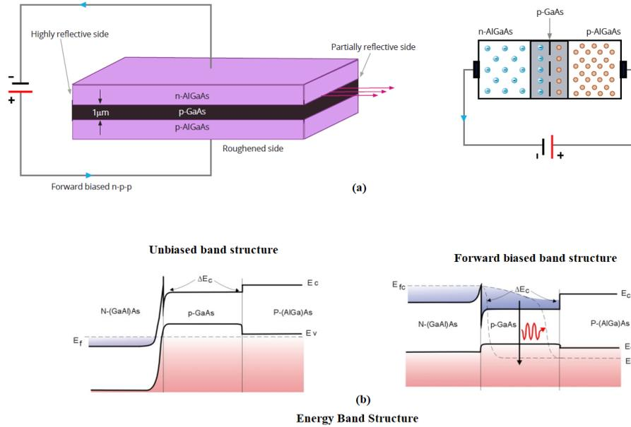
**Figure 9:** Hetrojunction laser
