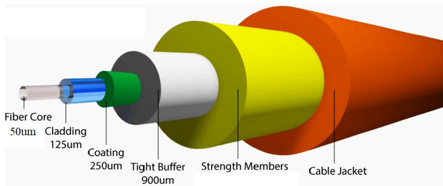
**Figure 11:** Typical optical fiber
