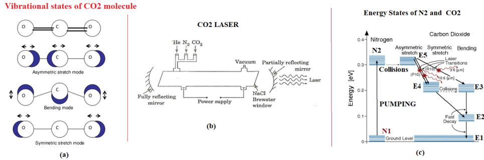
Figure 7: Vibrational modes of  $CO_2$  molecule
