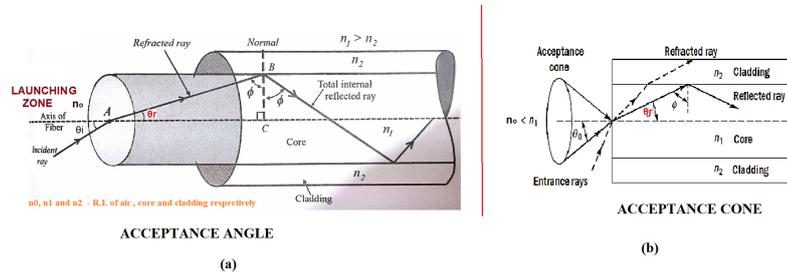
**Figure 13:** Propagation of light inside optical fiber
